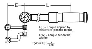
2. An attachment as shown below, is a drive extension which does not affect the torque and no correction is required. However, be careful when using a long extension to assure that the extension stays in line with the drive. You may support a long extension with your free hand with no measurable affects on the accuracy. Avoid using universal joints when torqueing unless the angle of mis-alignment is less than 5 degrees.
